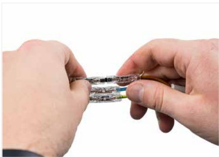
As an alternative to step 5: Strip 10 mm of conductor according to specification and set the connector (example shows staggered connectors).
