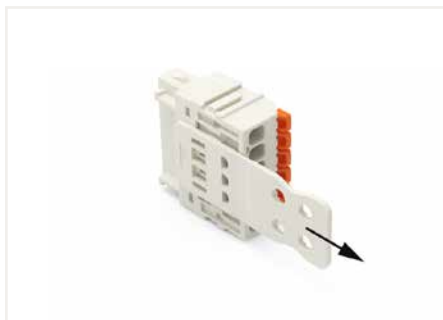
Insert the strain relief plate into the receptacle and pull until it hits the backstop in the conductor connection direction.
