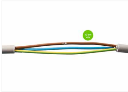
Strip the damaged cable approx. 10 cm uniformly around the damaged area.
