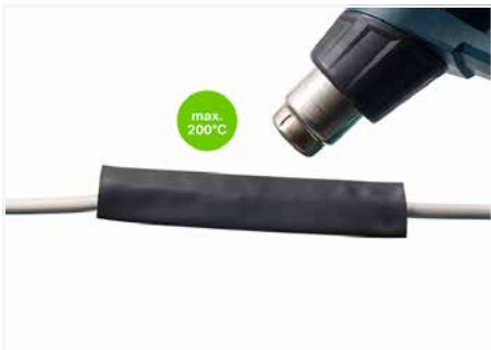
Heat the shrink tube evenly with a hot air blower between 110°C and 200°C.
