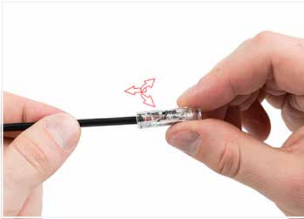
Twist the connector alternately left and right while pulling it off the conductor.
